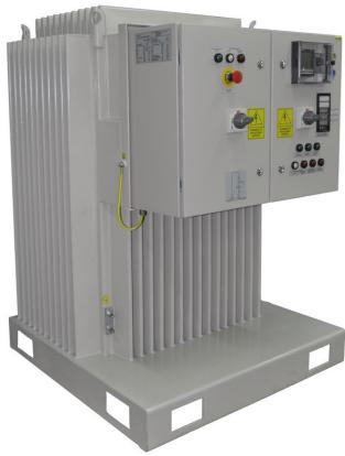
The transformer station type ST-T1/URB is a device designed for use on the ground with no explosion hazard. The transformer station ST-T1/URB is equipped with a power protections against short-circuits, overloads and lowered insulation resistance with installed transformer of rated power 63 kVA and upper rated voltage 400V.
